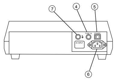
(1)Liquid Crystal Display16x1 character 9x7 dot matrix LCD display.(2)28Pin Test IC Socket(3)Keyboard(4)Fuse1A, protects tester from damage.(5)Power SwitchPower On or Off.(6)AC ReceptaclePlug power cord.(7)GNDGround
